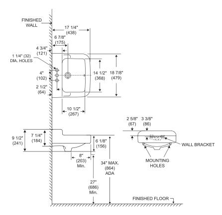
Dimensions may vary (+) or (-) 1/4". Dimensions shown in parentheses are in millimeters: 25.4 mm = 1 inch. Note: Fixture dimensions are nominal and conform with dimension and performance requirements of ASME/ANSI Standards A112.19.2M. Dimensions subject to change or cancellation without notice. Briggs is not responsible for the use of superseded or voided specification information.
