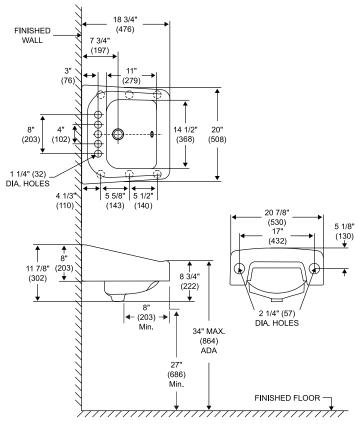
Dimensions may vary (+) or (-) 1/4". Dimensions shown in parentheses are in millimeters: 25.4 mm = 1 inch. Note: Fixture dimensions are nominal and conform with dimension and performance requirements of ASME/ANSI Standards A112.19.2M. Dimensions subject to change or cancellation without notice. Briggs is not responsible for the use of superseded or voided specification information.
