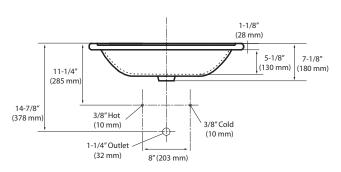
Dimensions may vary (+) or (-) 1/4". Dimensions shown in parentheses are in millimeters: 25.4 mm = 1 inch. Note: Fixture dimensions are nominal and conform with dimension and performance requirements of ASME A112.19.2-2008/CSA B45.1-08 standards. PSI rating: 20 minimum to 80 maximum per ASME A112.19.2-2008/CSA B45.1-08 standards. Dimensions subject to change or cancellation without notice. Briggs is not responsible for the use of superceded or voided specification information.
