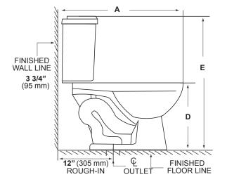
Dimensions may vary (+) or (-) 1/4". Dimensions shown in parentheses are in millimeters: 25.4 mm = 1 inch. Note: Fixture dimensions are nominal and conform with dimension and performance requirements of ASME A112.19.14. PSI rating: 20 minimum to 80 maximum per ASME A112.19.2. Dimensions subject to change or cancellation without notice. Briggs is not responsible for the use of superceded or voided specification information.
