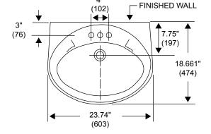
Dimensions may vary (+) or (-) 1/4". Dimensions shown in parentheses are in millimeters: 25.4 mm = 1 inch. Note: Fixture dimensions are nominal and conform with dimension and performance requirements of ASME A112.19.2-2008/CSA B45.1-08 standards. PSI rating: 20 minimum to 80 maximum per ASME A112.19.2-2008/CSA B45.1-08 standards. Dimensions subject to change or cancellation without notice. Briggs is not responsible for the use of superceded or voided specification information.
